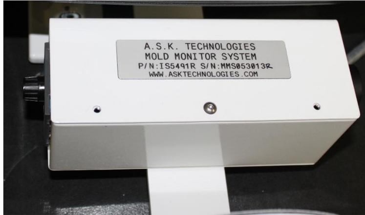
The remote control unit houses the main operator control components of the mold monitor system. This includes the power switch, timer, reset button, and a 6 pin plug for the cameras power/communication cable. The power switch and 6 pin plug are located on the back of the remote control unit while the timer is on the left and the reset button is on the right.
